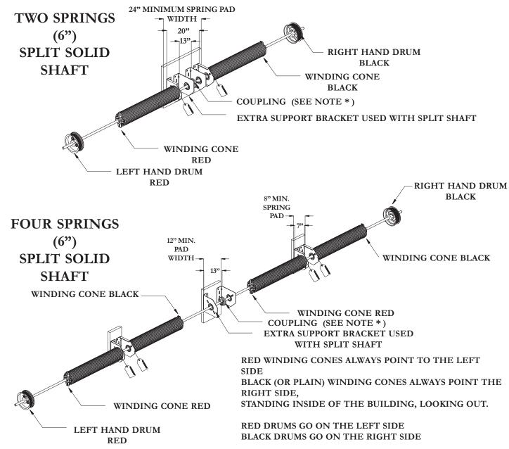
\*NOTE: COUPLING USED ON SOLID SHAFT ONLY. TIGHTEN CONNECTING BOLTS AFTER WINDING SPRING.
